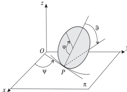
Figure 1: Generalized coordinates of a rolling disk.
