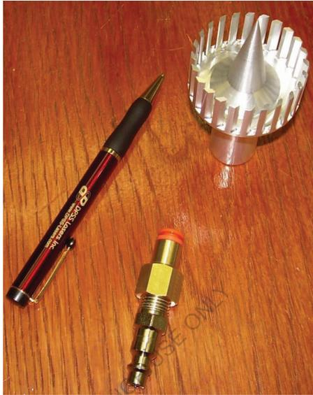
The following figures show to scale the various types and designs of aerodynamic foam generators or activators. Foam generators are also available in combination with accumulators and linear activators operating on the Bernoulli principle.
