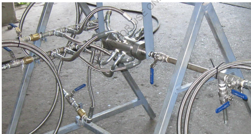
Industrial system for dynamic mixing and homogenization with maximal flow = 1000 liter per hour, under maximal pressure 30 bar
