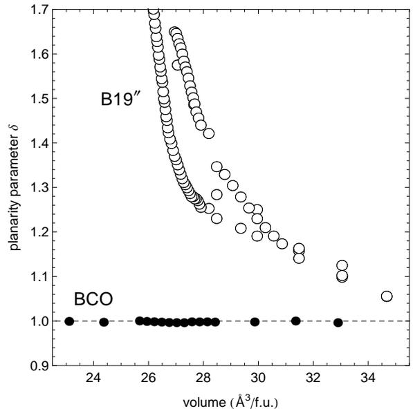
FIG. 6. The planarity parameter,  $\delta$ , describing the internal symmetry of the phases as a function of volume. The value of 1 found for the BCO phase indicates that the Ti atoms are located within the same atomic plane as the Ni atoms (see Fig. 1) and the internal geometry of the phase is too symmetrical. The B19'' values deviating from  $\delta = 1$  indicate an ability to store the shape information.
