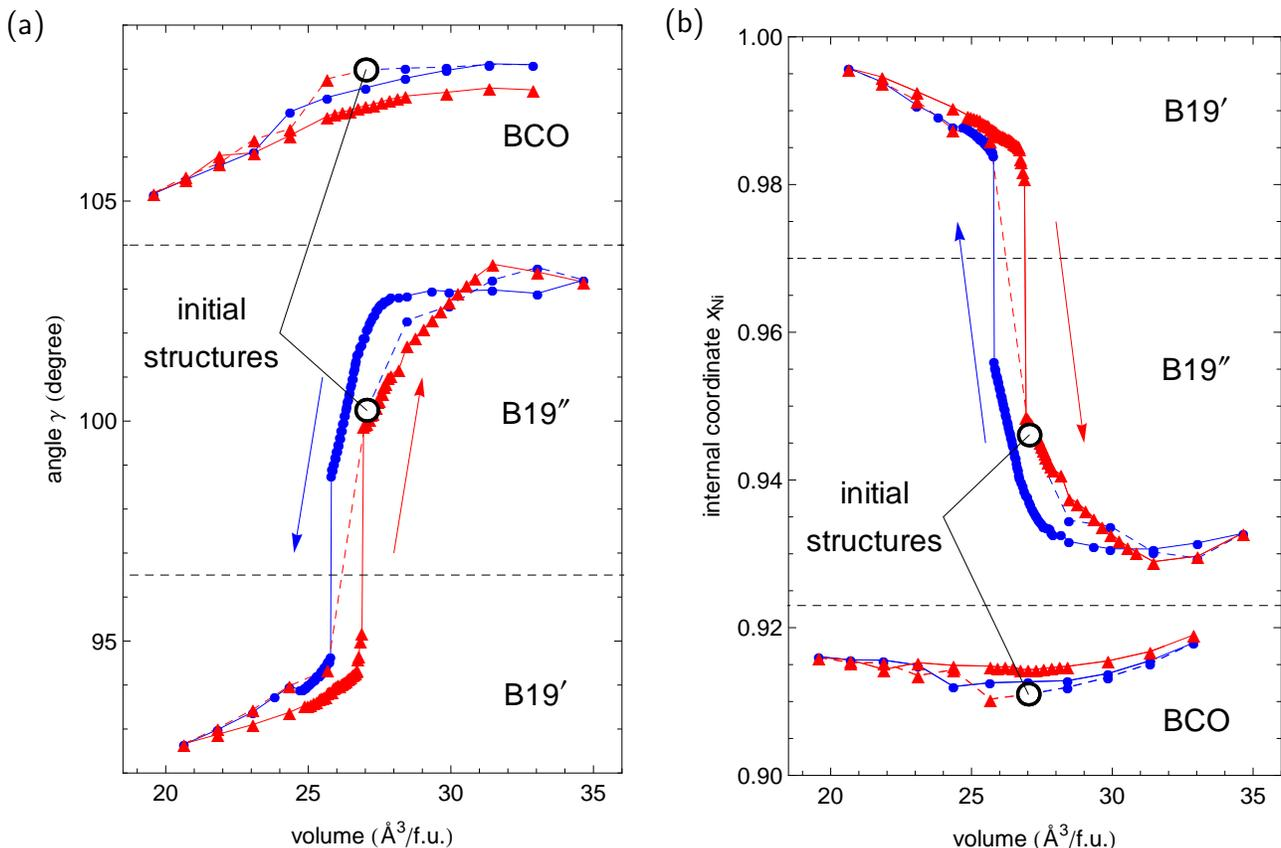
FIG. 2. Calculated dependence of (a) the monoclinic angle,  $\gamma$ , and (b) the internal coordinate,  $x_{\text{Ni}}$ , on the volume obtained from the QS simulations (see text). Along the B19' compression/decompression paths a region when an additional phase (B19'') becomes stable is found. Three ranges of monoclinic angle  $\gamma$ , that correspond (from the lowest values of  $\gamma$  to the highest) to B19', B19'' and BCO phases, respectively, are separated by horizontal dashed lines.
