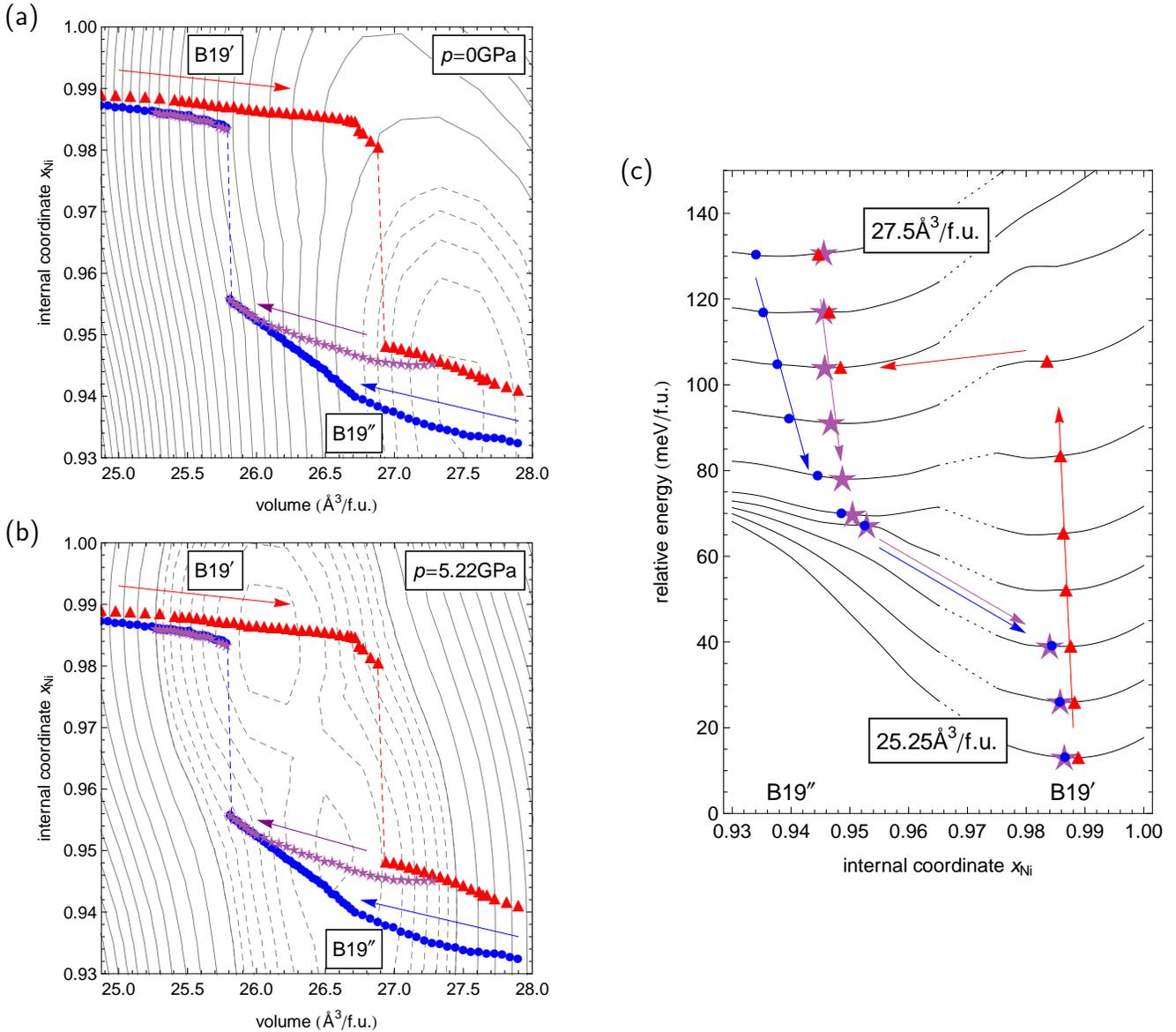
FIG. 3. Potential enthalpy surface for  $p = 0$  for fully relaxed states (a) and for  $p = 5.22$  GPa (b) along the reaction paths volume  $V$  and Ni internal atomic position  $x^{\text{Ni}}$ . The red, blue and violet symbols mark different volumetric loading conditions and corresponding trajectories (indicated by arrows). Part (c) shows vertical constant-volume cuts of the  $p = 5.22$  GPa enthalpy.
