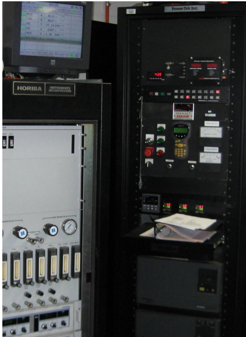
Figure 2, - the figure shows an example of a fragment of the location of the system of analytical and control equipment of the test bench, intended for testing and analytical evaluation of a diesel engine. Bench systems include elements of artificial intelligence and artificial neural networks. It is very important to show and disclose the novelty of using this system to achieve an ideal end result or its equivalent in relation to the claimed material, as well as to show the interaction of the control and analytical components of the system with elements of artificial intelligence
