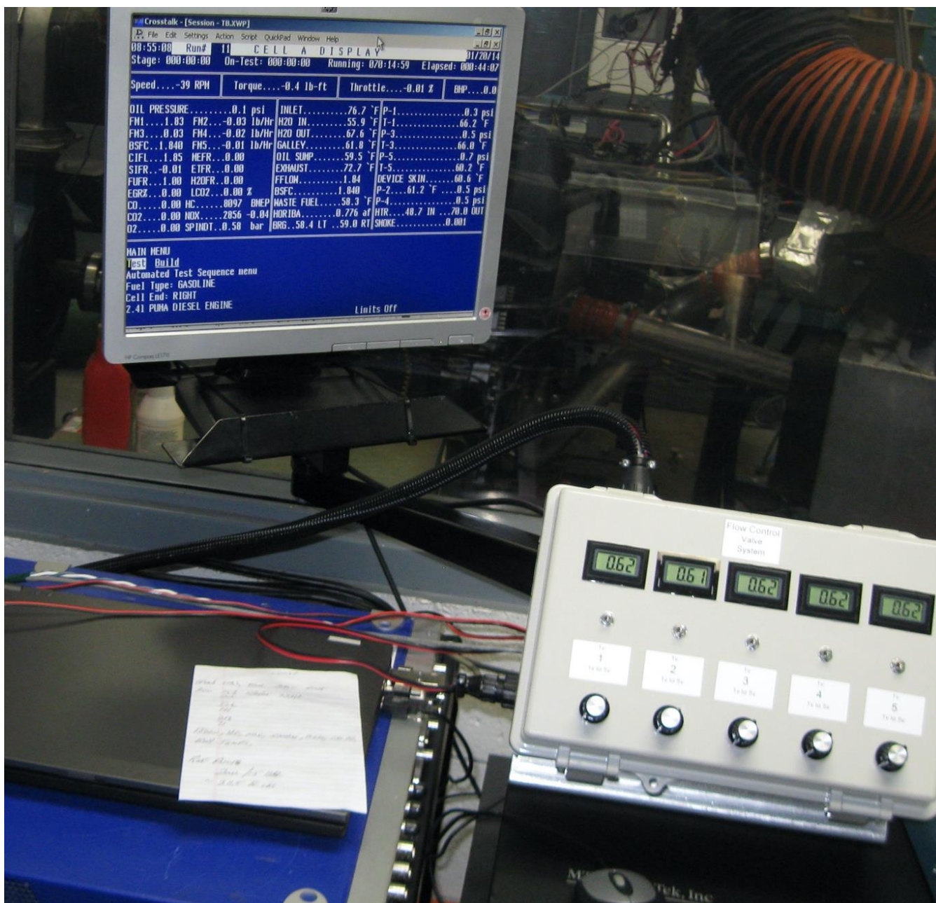
Figure 3, - the figure shows an example of the location of the system of analytical and control equipment of the test bench, intended for testing and analytical evaluation of a diesel engine. Bench systems include elements of artificial intelligence and artificial neural networks. It is very important in the application materials to show and disclose the novelty of the application of this system to achieve an ideal end result or its equivalent in relation to the claimed material
