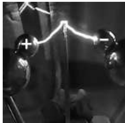
Figure 6: Photo of an electrostatic spark over a glass pane.
